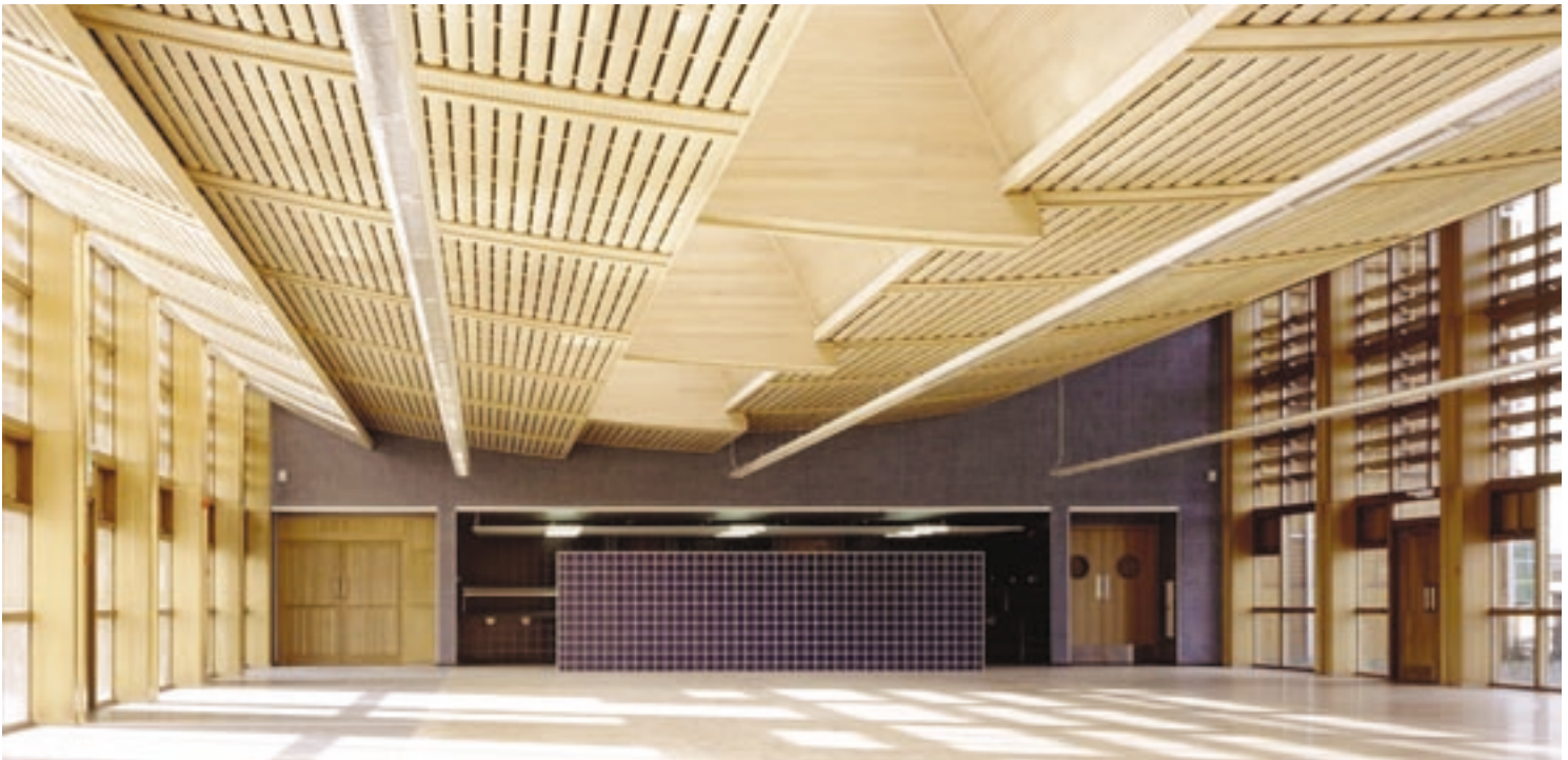
Ninety-eight percent of the materials in this European Commission building outside Dublin are re-useable or recyclable. Opened in 2002, it has won numerous sustainable building awards. Ceiling slats are American ash. Architect: Ciaran O'Connor, Office of Public Works.
